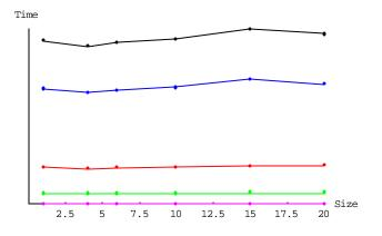
Figure 15: The effect of multiple polygons. 60 random vertices are divided into several polygons and triangulated. The horizontal axis is the number of polygons.
