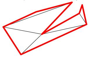
Figure 1: A triangulated polygon. The red edges are edges of the polygon, the black lines are the diagonals introduced.
