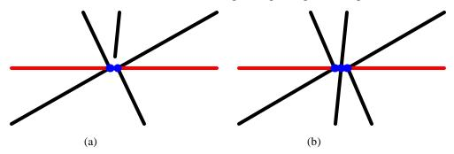
Figure 10: Multiple intersection of edges: (a) just before intersection and (b) just after intersection. Only one new point has been introduced. Note that all three points have the exact same coordinates.
