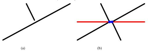
Figure 8: Intersection of edges: (a) just before intersection and (b) just after intersection. Two new points have been introduced, and regions on both sides have been split. Note that the two points have the exact same coordinates.
