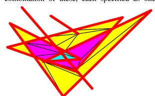
degeneracies between them. The output of the routine is a set of triangles, each one with its own depth, the three vertices of the triangles being either vertices from the input, or points where edges intersect.
