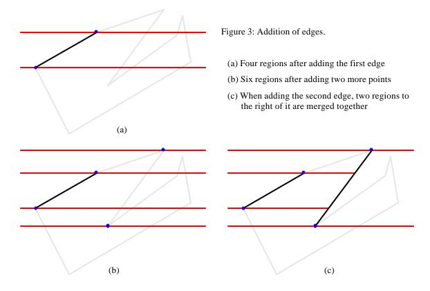
defined. When the algorithm has split one region during the addition of an edge, it needs to find the correct region below to move into. If there is only one region, this is trivial, if there are two, then the correct one can be found by checking whether the endpoint of the edge being added is to the right or left of the edge that separates the two regions.
