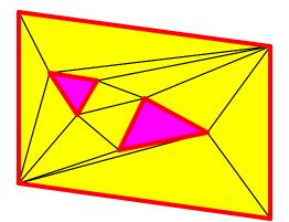
Figure 6: Triangulation of multiple polygons with varying triangle depth. Yellow is depth 1, and magenta is depth 2.
